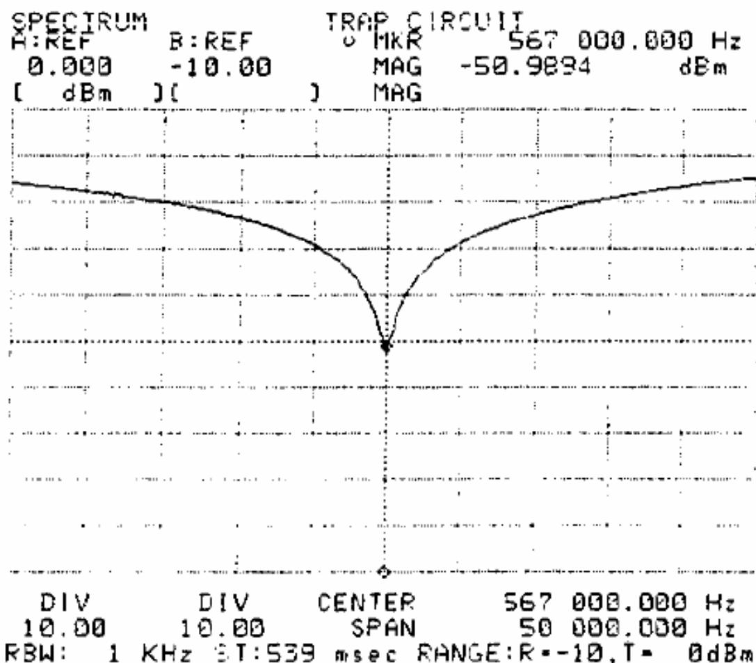
**MW- diplexer Murcia ( Spain ) 567 kHz, 25 kW - 855 kHz, 300 kW**
